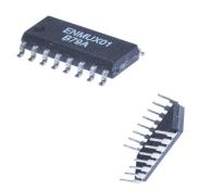
The multiplexer chip (MUXC01) is designed to select the passage-path of the digital signals between one input and nine outputs. It is mainly composed of a basic 9-bit shift register (nine cascaded D-flip-flops) and nine 2-input AND gates (see Figure 2).
